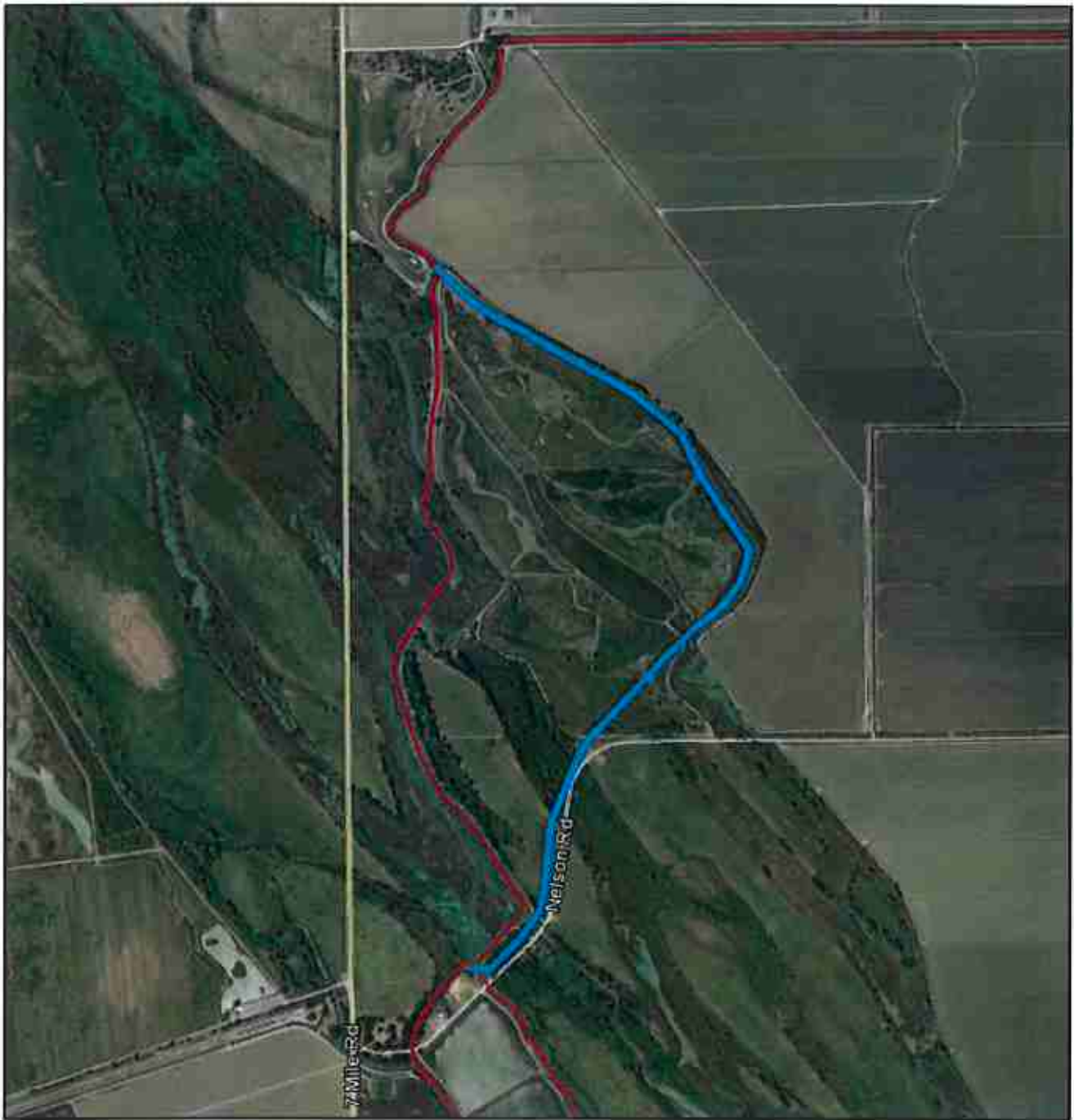
Figure 3. Overview of Existing Canal Alignment (Red) and Conceptual Alignment (Blue) of Reservoir Bypass Canal.
